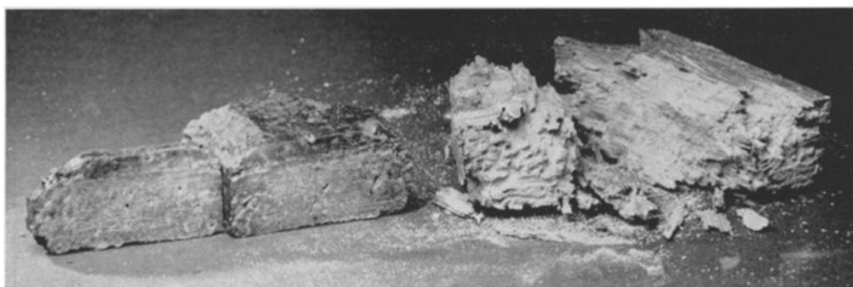
FIGURE 5 Samples of wood taken from crosspiece of Coronation Panel (right: untreated; left: treated by wax immersion)
