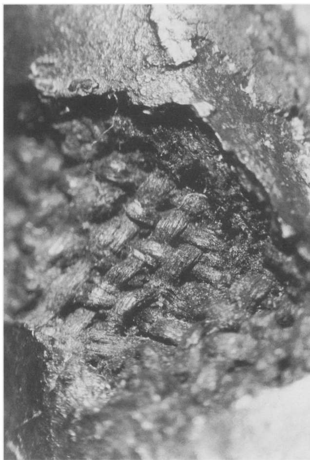
Fig 8. Magnified close-up of the cloth on the shoulder of the Walters Buddha (pl. I and fig. 1). The plain weave structure is readily apparent. The saturated fibers are well preserved in the lacquer. (25x)
