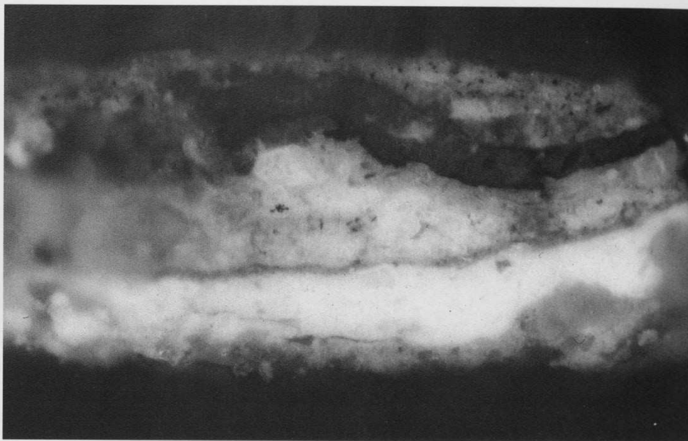
Fig. 8. Paint cross section from the hair of Head A. This sample contains an original ochre ground and four paint layers (78x magnification).
